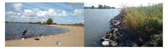
Figure 4 - Preparing the location; white buckets used to mark the spots for sampling; Locations like the one on the right were avoided due to the difficulty in safely operation the spectrometer on them.
